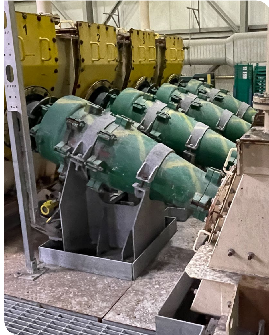
Image: Dense Media Separation (DMS) cyclone - Stage 1 DMS at Renard
