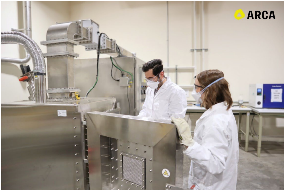
Figure 2. Arca scientists working with microwave activation technology accelerating carbon dioxide removal in mine waste at their Vancouver laboratory
