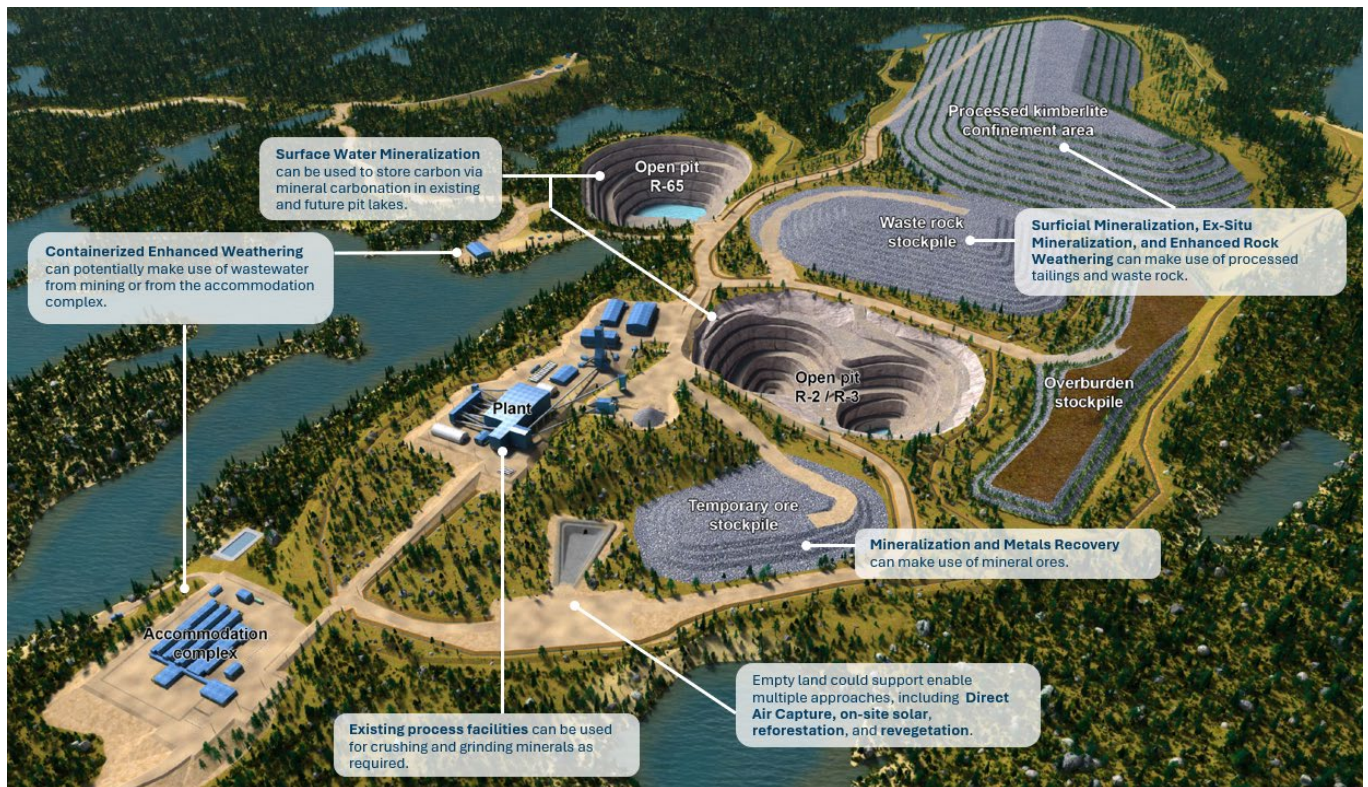
Figure 1. Schematic view of the Renard site showing existing infrastructure and CDR techniques being investigated as part of the Decarbonisation Strategy.
