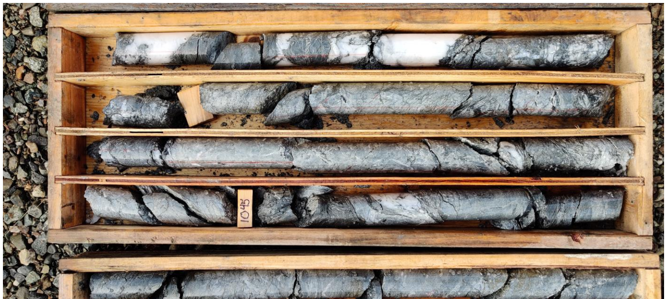
Figure 4: Drill core from the zone of silicification, quartz veining and brecciation in LC20-06 at Sidewinder Blowout.
