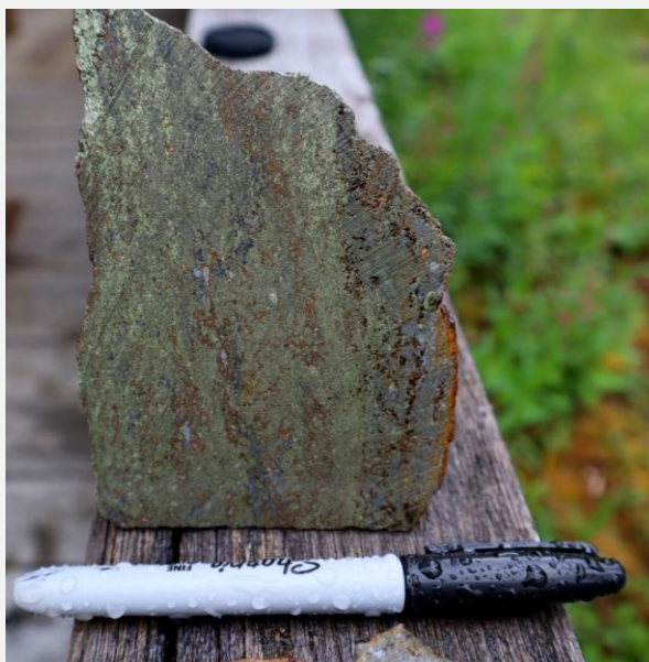
Figure 1: Photo of the massive sulphide float (dominantly chalcopyrite with minor galena) from the Kiwi prospect.
