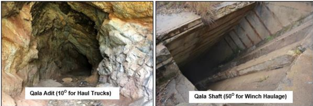
Image 2: Qala Adit and Qala Shaft will provide access to the Kimberley East underground target.
