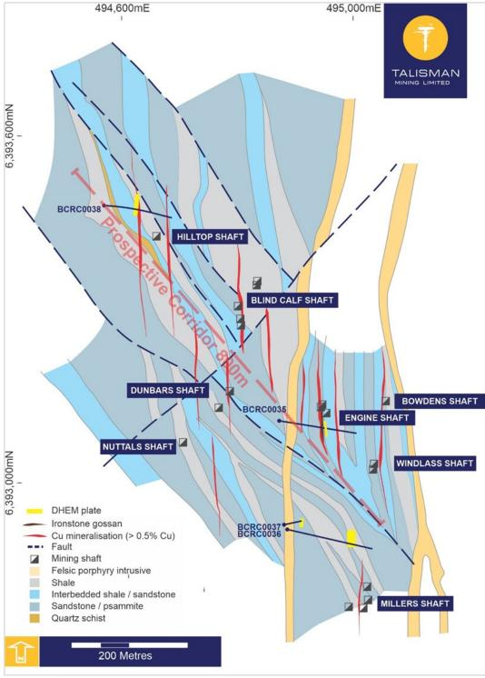
Figure 2: Blind Calf Prospect geological interpretation showing recent drilling and tested DHEM conductors.
