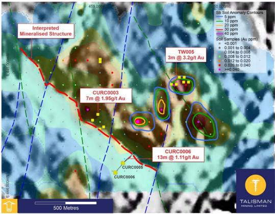
Figure 5: Cumbine Gold Prospect showing previous drilling<sup>4</sup>, soil geochemistry and recent RC drilling.
