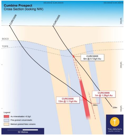
Figure 4: Cumbine Gold Prospect cross-section (looking NW), showing holes CURC0005 and CURC0006.
