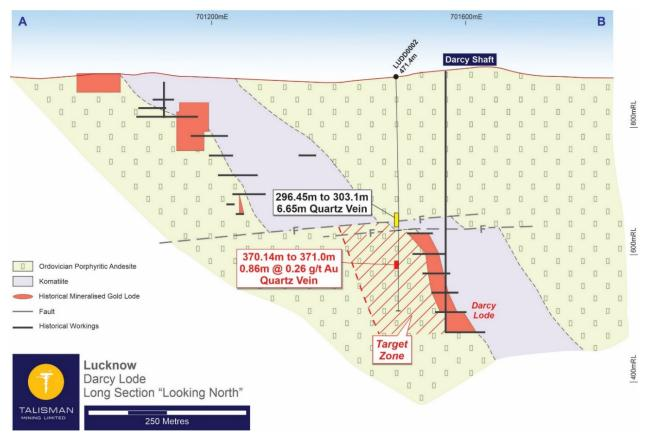
Figure 7: Long-section view (looking north) through Darcy Lode showing interpreted pierce point of hole LUDD0002.
