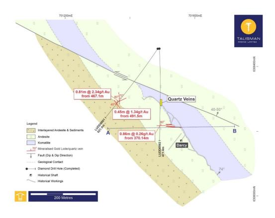
Figure 8: Composite plan view (600mRL), showing interpreted geology and completed TLM drill holes.
