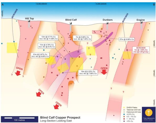
Figure 3: Blind Calf Prospect long-section showing mineralised lenses and DHEM targets<sup>4</sup>.
