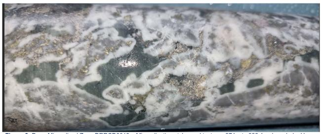
**Figure 8:** Deep Mineralised Zone DRRCD0019 – Mineralisation styles and textures 374m to 399.1m down-hole. Upper Panel (field of view 27cm) – Massive sphalerite (25%), quartz breccia (25%), galena (50%). Lower Panel (Field of view 16cm) – Chalcedonic vein textures with interstitial Chalcopyrite (2%-3%), pyrite (3%-5%). Refer Table 1 for Mineral abundance estimates. See Note 1.
