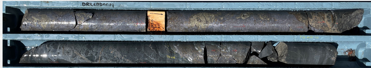
DRRCD0019 - Massive Pb-Zn Sulphides 1.7m at 26.5% Pb, 7.8% Zn, 558g/t Ag, 0.7% Cu and 0.81g/t Au from 224.5m
