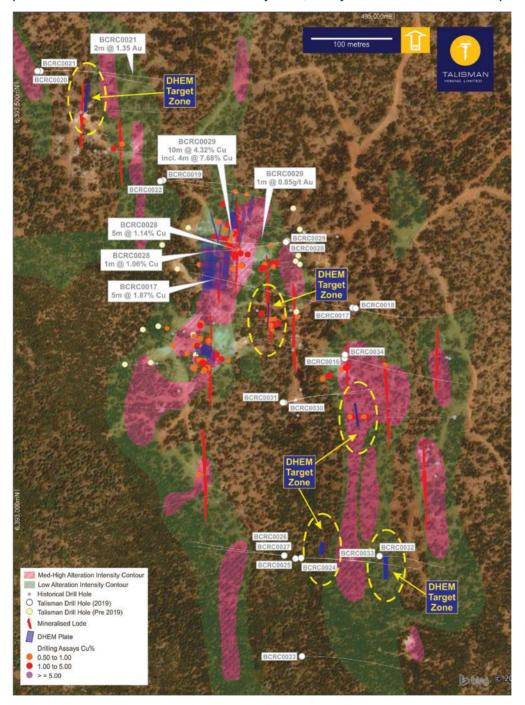
Figure 3: Blind Calf Prospect collar plan showing selected TLM<sup>5</sup> and historic intersections, highlighting new proximal drill-ready target areas.
