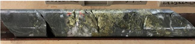
Figure 5: Blind Calf Prospect – BCDD003: Brecciated quartz & semi-massive chalcopyrite sulphide vein
