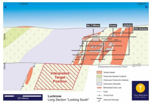
Figure 3: Lucknow Project interpreted long section, showing the interpreted faulted offset mineralisation target position.
