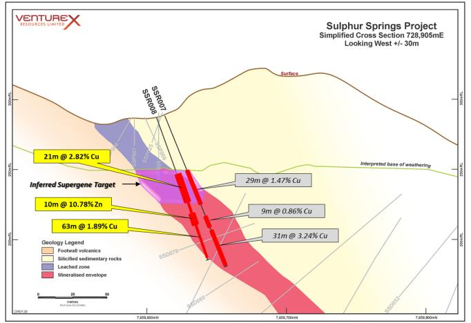
Figure 1: Cross-section on 728,905mE showing location of holes SSR007 and SSR008
