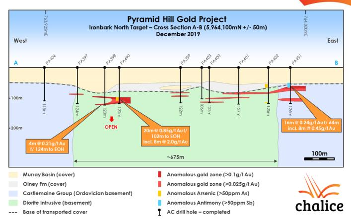
Figure 3. Ironbark North Target Cross Section A-B (5,964,100mN +/- 50m).
