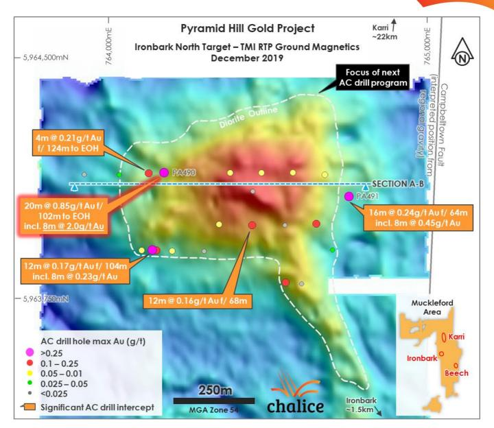
Figure 1. Ironbark North Target Plan View – Maximum gold in AC drilling over Total Magnetic Intensity (TMI) Reduced to Pole (RTP) ground magnetics.
