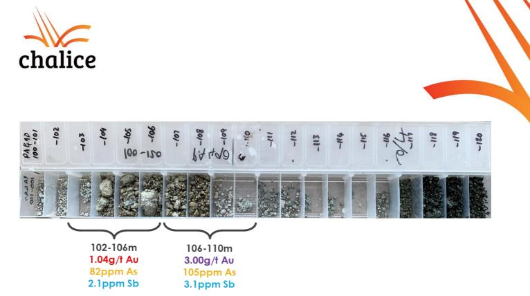
Figure 2. AC drill chips and significant assay results from PA490 – interval from 100m to 120m.
